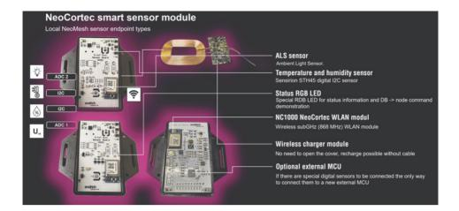
local WLAN sensor module built around the NeoCortec MESH modem. This module is optimized for battery operation, featuring wireless charging for the on-board lithium polymer cell. The product exists with optimal low power consumption using the internal ARM Cortex M0+ MCU built in to the NC1000 mesh module, other version offers an external low power MCU and a further feature connector for external I<sup>2</sup>C and analogue sensors.
