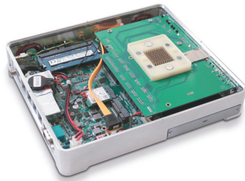
5 | Docking station PC: 100 pole docking-connector on the top of the housing, inside the main board organization can be reviewed
