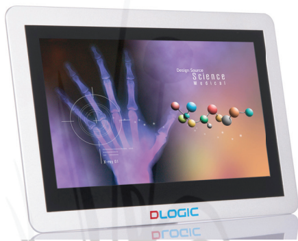
3| SDM: ARM based smart display boards with LINUX operating system, offering many industrial interfaces and built in touch panel
