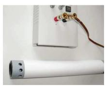
applying music on the speaker, we can hear thinner sound. The high pressure in front of the membrane and the low pressure behind it will generate acoustic wind; the waves will find the shortest path through the holes. In order to make its way longer, we can cover the holes by a paper roll, and the perceived sound becomes immediately much richer.
